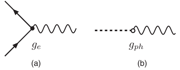
FIG. 1. Feynman diagrams for the vertices in Eq. (23), coupling the field \varphi (wiggly curve) to (a) electrons (solid line) and to (b) phonons (dashed). The Coulomb (piezoelectric) vertex \sim g_e ( \sim g_{ph} ) is shown as filled (open) circle.
