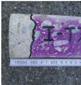
Figure 9. Concrete carbonation depth assessment.
