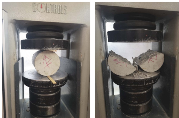
Figure 6. Splitting concrete tensile strength test.
