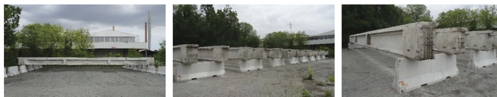
Figure 1. PC bridge deck beams stored at the testing site.
