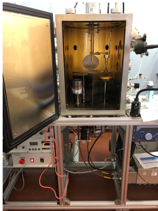
Fig. 4.7 Homebuilt RF sputtering system used for the gold deposition
