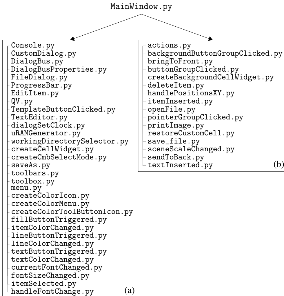
Fig. 5.2 Contents of the MainWindowItems folder. (a) Dialogs, progress bars, and graphical widgets and elements. (b) Python files performing specific routines or functions related to the graphical part.
