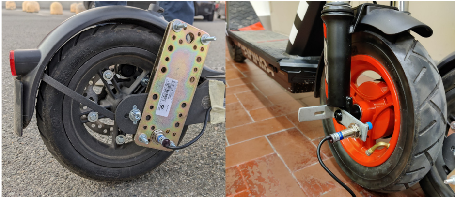
Figure 110 - Proximity sensor mounted on the rear wheel of Xiaomi Pro II and on the front wheel of Aprilia ESR2
