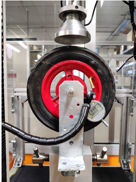
Figure 19 - Clamping system and dial indicator on the wheel hub
