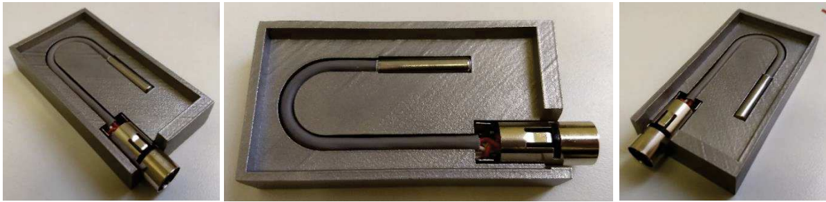
Figure 3: Installation of the sensor with cable and connector into the simulator reproducing the core element.
