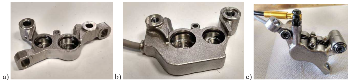
Figure 9: Brake caliper after mechanical tooling (a, b) and in the final assembled configuration (c).
