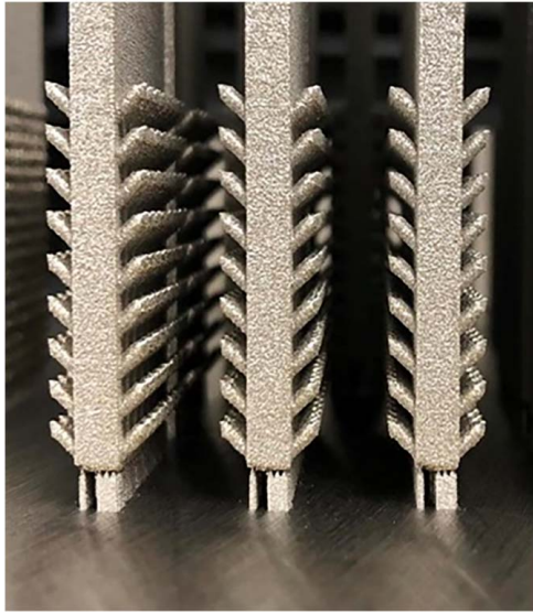
Fig. 7 As-built samples with down-oriented spiked cylinder anchors. No supports are provided in this case since anchors orientation is sufficient to guarantee self-supporting. The same condition occurs for pyramids and other oriented spiked anchors.
