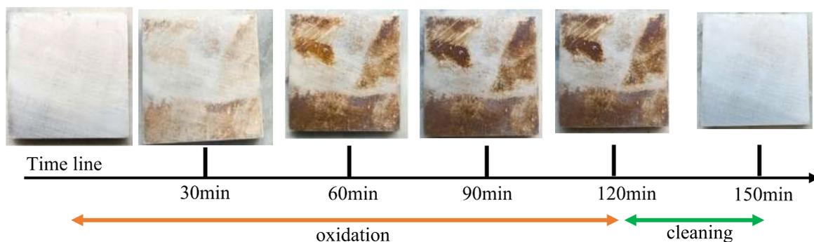
Fig. 3. Photographs of samples at increasing values of immersion time in potassium permanganate solution (30 min, 60 min, 90 min, 120 min) and after 30 min of oxalic acid immersion. Each sample is  $30 \times 30 \times 5 \text{ mm}^3$ .
