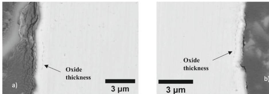
Fig. 6. Two SEM images of the left (a) and right (b) borders of the sample immersed for four hours in a pH 5 solution with a permanganate ion concentration of  $6 \cdot 10^{-5}$  mol/l. On micrograph, the oxide layer is highlighted. Both images were acquired using the Backscattered Electrons detector.
