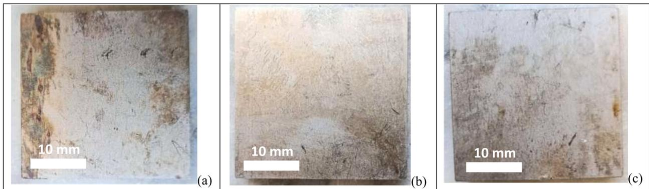
Fig. 4. Results of the second set of immersion tests: sample immersed for 4 h in the solution with concentration  $[\text{MnO}_4^-] = 3 \times [\text{H}^+]$  and with  $\text{pH} = 4$  (a) or  $\text{pH} = 5$  (b), and in the solution with concentration  $[\text{MnO}_4^-] = 6 \times [\text{H}^+]$  and with  $\text{pH} = 5$  (c).
