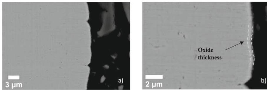
Fig. 5. Two SEM images (a & b) of the sample immersed for four hours in a pH 5 solution with ion concentration permanganate equal to  $10^{-5}$  mol/l. Both images were acquired using the Backscattered Electrons detector.
