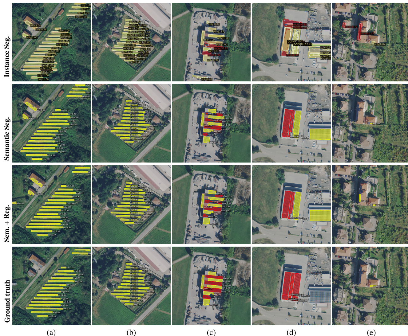
FIGURE 7. Qualitative results of our best solutions on four different installations, including industrial plants with different scales and domestic PV panels. From top to bottom: instance segmentation, semantic segmentation, semantic segmentation with post-processing polygonization and regularization algorithm, initial ground truth. Best viewed on screen.
