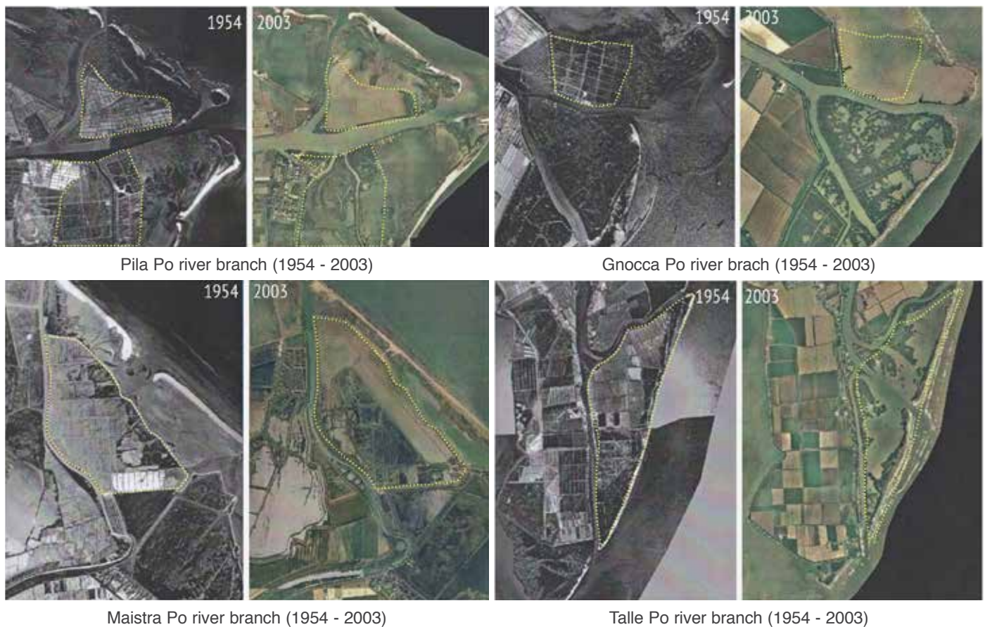
Figure 3. Examples of the widespread erosive retreat affecting the Po Delta coastline.
