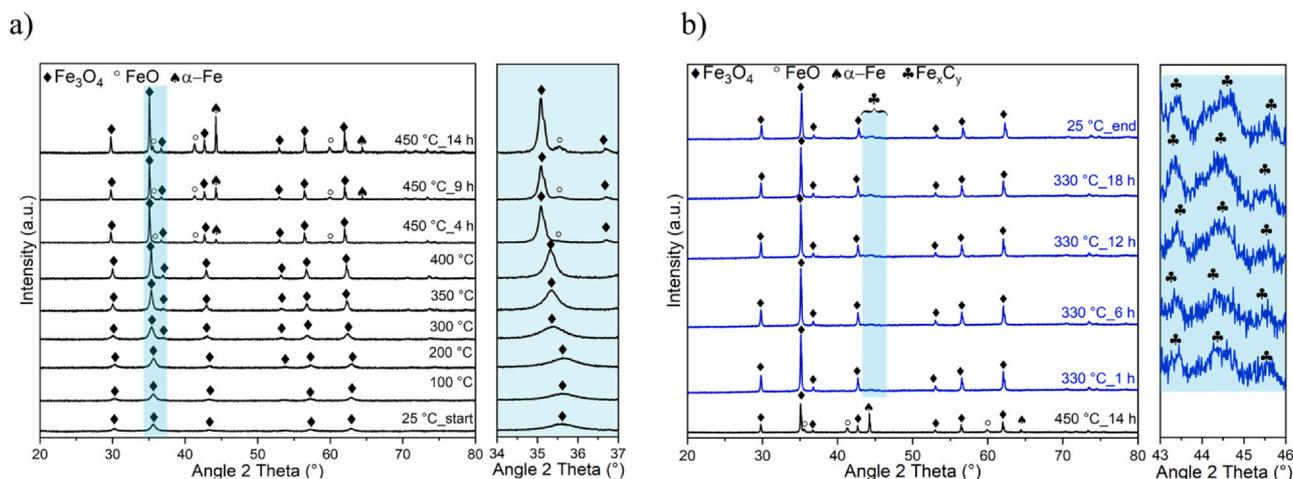
**Fig. 5** – In situ XRD patterns of fresh  $\text{NaFe}_3\text{O}_4\text{-CP}$  catalytic powder under reducing atmosphere a)  $\text{H}_2/\text{Ar}$  from  $25^\circ$  to  $450^\circ\text{C}$ , black profiles; b)  $\text{H}_2/\text{Ar}$  at  $450^\circ\text{C}$  for 14 h, black profile and  $\text{H}_2/\text{CO}/\text{N}_2$  at  $330^\circ\text{C}$  for 18 h, blue profiles.
