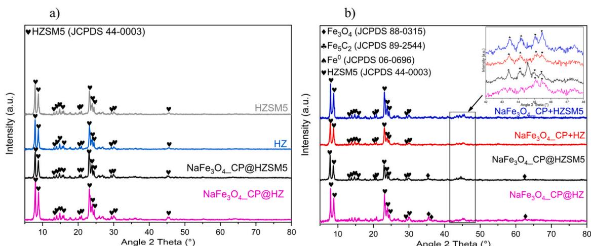
**Fig. 4** – XRD patterns of (a) fresh zeolites and core-shell structures and (b) spent granule mixed catalysts and core-shell structures.
