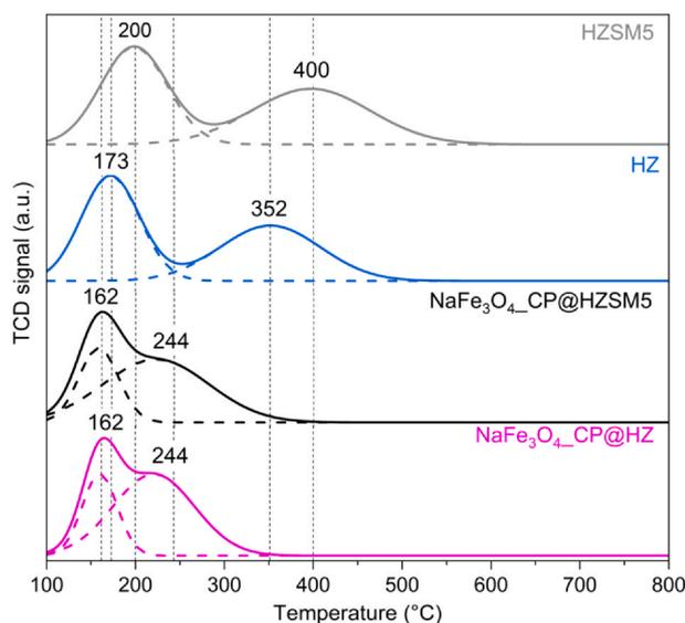
Fig. 7 –  $\text{NH}_3$ -TPD fresh catalysts profiles.
