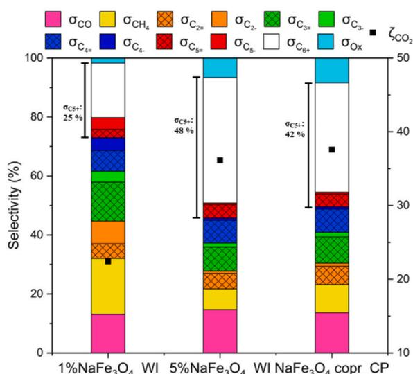
**Fig. 12** – Comparison catalytic performance of 1%  $\text{NaFe}_3\text{O}_4\text{-WI}$ , 5% $\text{NaFe}_3\text{O}_4\text{-WI}$  and  $\text{NaFe}_3\text{O}_4\text{-CP}$  catalysts at 330 °C. Reaction conditions: 2.0 MPa, 21.96  $\text{NL}\cdot\text{gFe}_3\text{O}_4\text{-h}^{-1}$ , TOS = 14 h.
