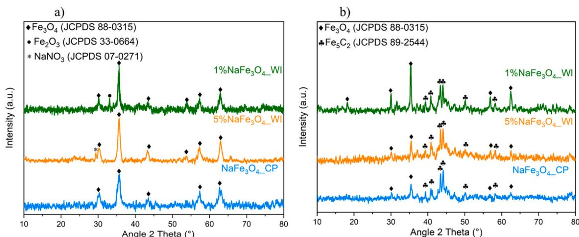
**Fig. 3 – XRD patterns of the (a) fresh and (b) spent Fe<sub>3</sub>O<sub>4</sub>-based catalysts: 1%NaFe<sub>3</sub>O<sub>4</sub>\_WI, 5%NaFe<sub>3</sub>O<sub>4</sub>\_WI and Na-Fe<sub>3</sub>O<sub>4</sub>\_CP.**
