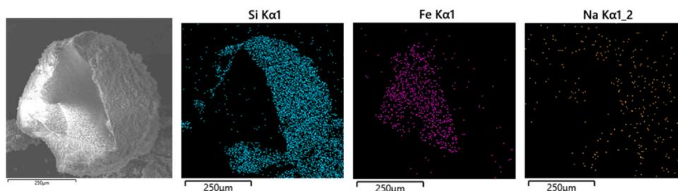
Fig. 8 – FESEM-EDS images of the sample:  $\text{NaFe}_3\text{O}_4\text{-CP@HZSM5}$ .
