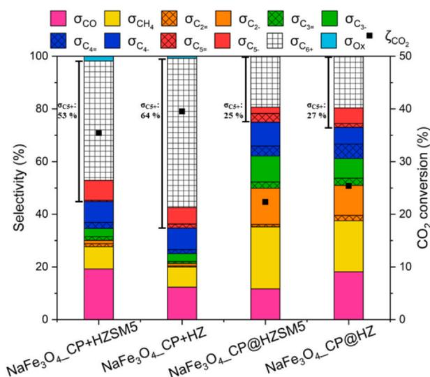
**Fig. 13** – Comparison of catalytic performance among physical mixture and core-shell of  $\text{NaFe}_3\text{O}_4\text{-CP}$  with commercial and homemade hierarchical zeolite. Reaction conditions: 330 °C, 2.3 MPa, and a flow rate of 21.96  $\text{NL}\cdot\text{gFe}_3\text{O}_4\text{-h}^{-1}$  TOS= 14 h.
