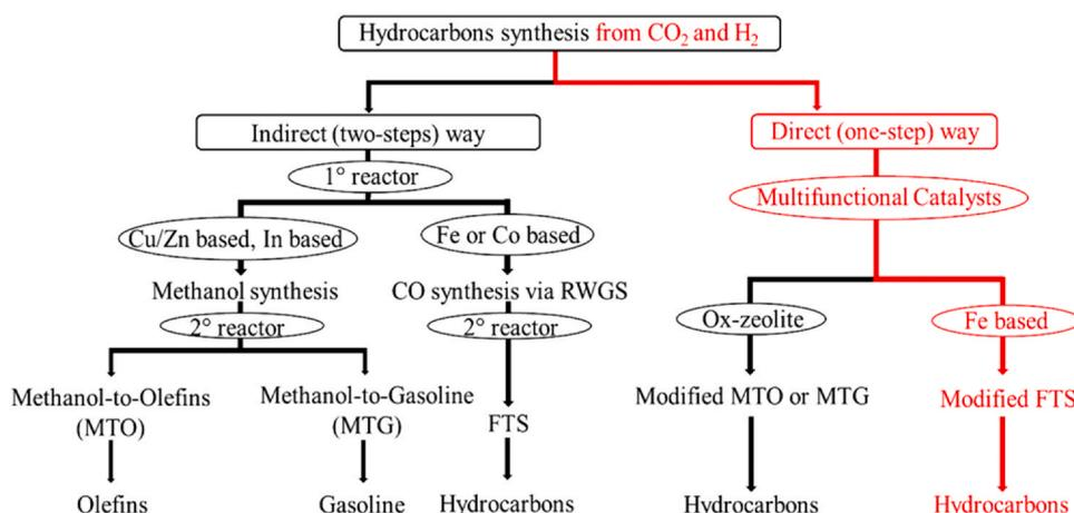
Fig. 1 – Different ways to hydrogenate CO<sub>2</sub> to hydrocarbon final products.
