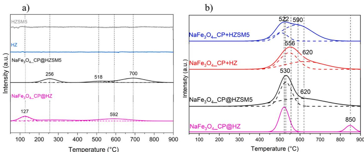
**Fig. 10** – CO<sub>2</sub>-TPD profiles a) fresh core-shell catalysts and their counterpart zeolite; b) spent core-shell structures and physical mixture.
