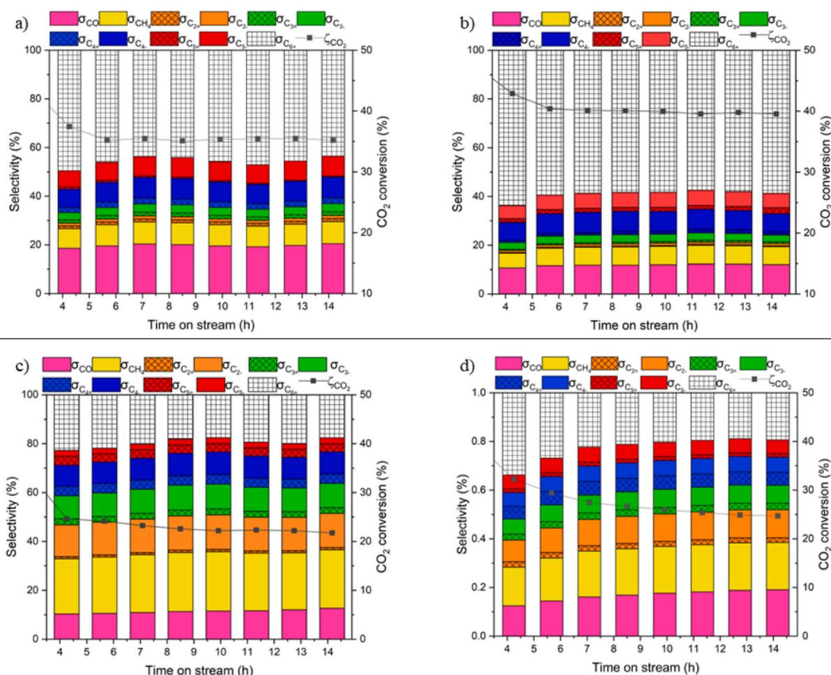
**Fig. 14** – Time-on-stream (TOS) tests up to  $\approx 14$  h, temperature:  $330$  °C, pressure:  $2.3$  MPa, and flow rate:  $22 \text{ NL} \cdot \text{g}_{\text{Fe}_3\text{O}_4}^{-1} \cdot \text{h}^{-1}$  with an inlet  $\text{H}_2/\text{CO}_2/\text{N}_2$  molar ratio equal to  $15/5/3$ : a)  $\text{NaFe}_3\text{O}_4\text{-CP+HZSM5}$ ; b)  $\text{NaFe}_3\text{O}_4\text{-CP+HZ}$ ; c)  $\text{NaFe}_3\text{O}_4\text{-CP@HZSM5}$ ; d)  $\text{NaFe}_3\text{O}_4\text{-CP@HZ}$ .
