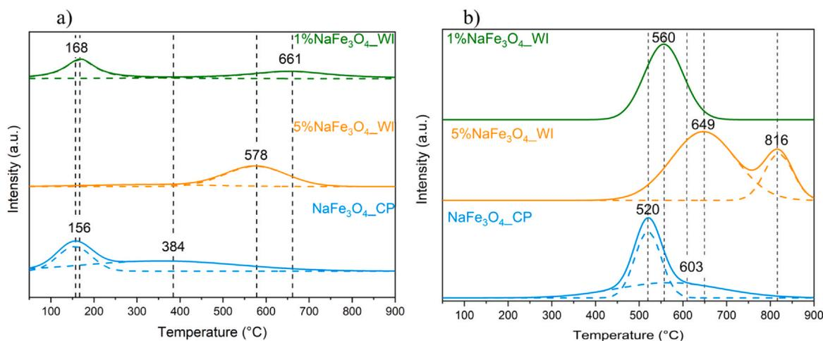
Fig. 9 –  $\text{CO}_2$ -TPD profiles a) fresh iron-oxide and b) spent iron-oxide samples.
