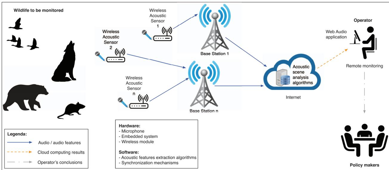
Fig. 6. Diagram of a WASN for wildlife monitoring.
