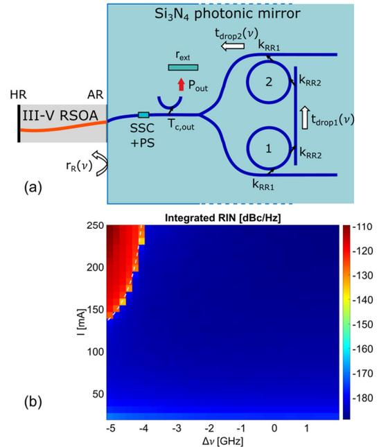
Fig. 1. Schematics of the III-V/SiN hybrid laser (a) and integrated RIN for different detuning  $\Delta\nu$  of lasing frequency and RSOA bias current (b).  $\Delta\nu=0$  corresponds to lasing at the reflectivity peak, which is centered at 1310 nm.
