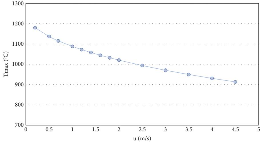
FIGURE 20: Maximum receiver temperature based on wind speed.
