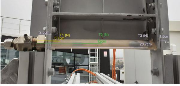
FIGURE 3: Focal plane and position of N-type thermocouples.
