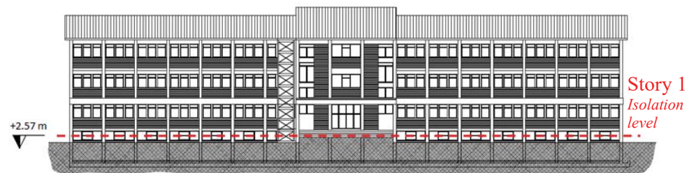
Figure 8. Position of the isolation level (red dashed line) with location of the single-concave FP devices.
