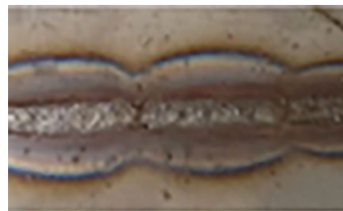
Fig. 19 SMAW bead surface
