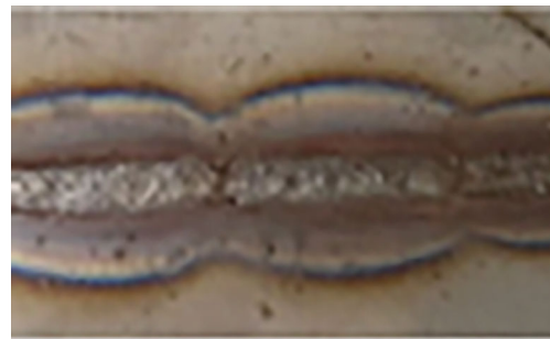
Fig. 19 SMAW bead surface
