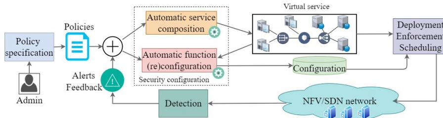
Fig. 2. Full workflow of automated virtual network configuration
