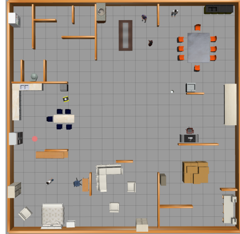
Fig. 3: Example of indoor environment in Gazebo where navigation policies can be trained or tested, accessing different areas with realistic obstacles and narrow passages. A Jackal UGV has been spawned to reach the goal (red circular target).
