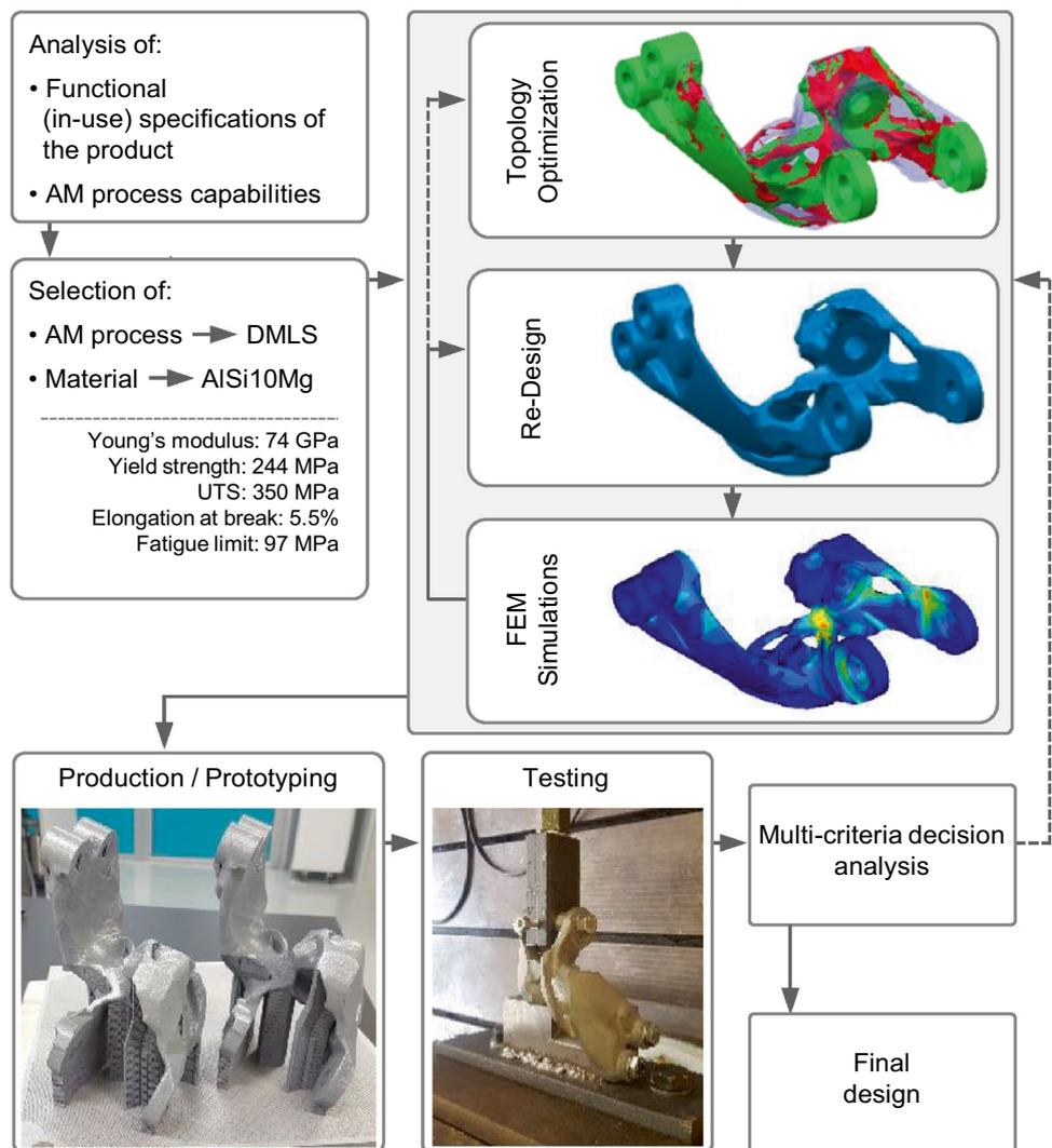
The bracket made of AlSi10Mg and re-designed for AM led to a 69%-mass reduction (i.e.,  $k=0.31$ ), with respect to the bracket made of cast iron and conventionally manufactured. Moreover, the bench tests conducted on the additively manufactured prototype highlighted a significant improvement in performance of all the acceptance criteria [56].
