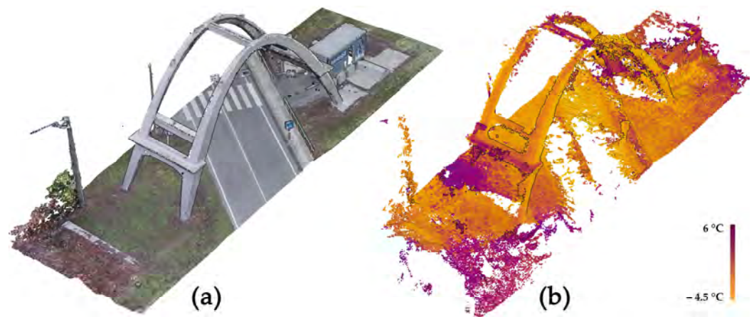
Figure 14. (a) Photogrammetric dense point cloud derived from the images acquired from the DJI Zenmuse XT2 visible sensor; (b) photogrammetric dense point cloud derived from the TIR images acquired from the DJI Zenmuse XT2 thermal sensor.
