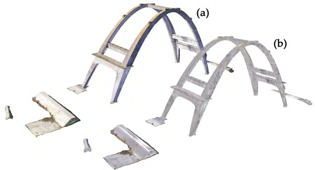
Figure 7. (a) Photogrammetric 3D mesh of the arch with the original texture; (b) reprojection of the edited texture on the original photogrammetric 3D mesh.
