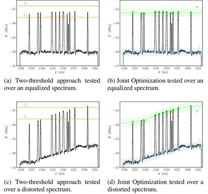
**Fig. 1:** In (a) all the channels appear as peaks in the spectrum having the same power level (equalized), whereas in (c) the spectrum becomes distorted and the channels are no more equalized. While in (a) the thresholds  $T_H$  and  $T_L$  (colored orange) can successfully separate channels from anomalies, in (c) the use of thresholds becomes ineffective. Figures (b) and (d) depict the channel and ASE trends,  $\nu$  and  $\mu$ , estimated by our proposed method.
