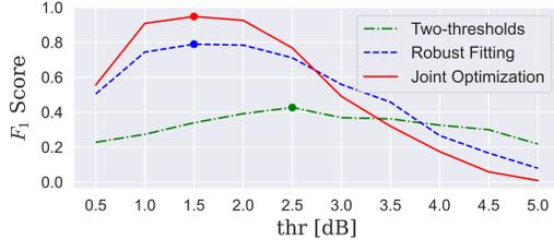
**Fig. 2:**  $F_1$  Score vs. inlier thresholds. For each method, we selected the threshold value leading to the highest  $F_1$  Score. The two-threshold approach achieves a maximum  $F_1$  Score of 0.42 at 2.5 dB. The robust fitting approach and our joint optimization use a threshold of 1.5 dB, achieving  $F_1$  Scores of 0.79 and 0.95, respectively.
