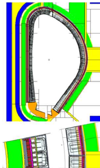
Figure 3. WCLL DEMO MCNP model: poloidal section showing the inboard and outboard breeding blanket ( top ) and toroidal section along the equatorial plane ( bottom ).
