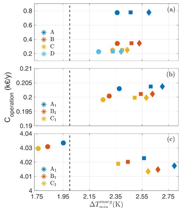
**FIGURE 12.** Operation cost estimated for the CS3U2 feeder (a), PF61 feeder (b) and TF jumper (c), respectively, reported as a function of the computed minimum temperature margin during the investigated plasma pulse, for different configurations and operating mass flow rate values: circle 2 g/s, square 5 g/s, diamond 10 g/s, respectively. The value of  $\Delta T_{min}^{CS}$  is also reported (dashed line).
