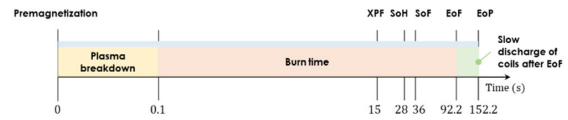
FIGURE 4. Timeline of the standard SN plasma operating scenario considered in the present analysis.
