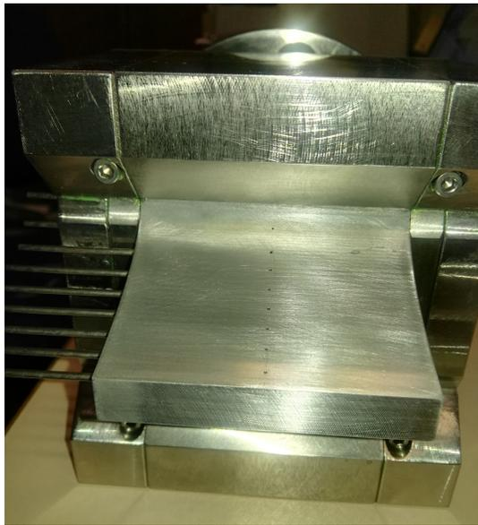
Fig. 4. Pressure ports on the nozzle plug wall.
