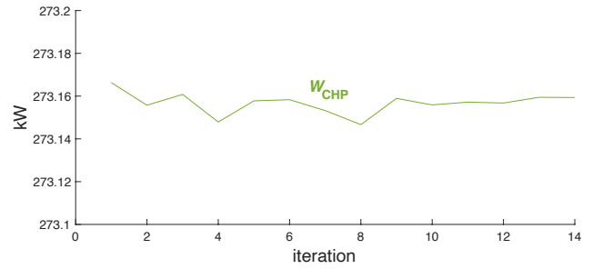
Fig. 8. Zoom of the variations in the CHP electrical output during the iterative process in the summer case at hour 18.
