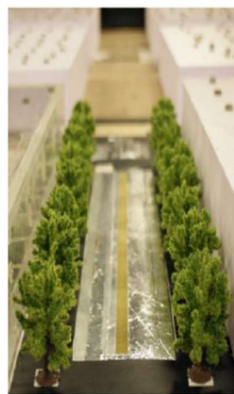
Figure 1: (a) Scheme of the wind tunnel (left): 1 test section; 2 heat exchanger system; 3 fan; 4 diverging system; 5 converging system and generating turbulence grid. Street network simulated inside the test section (right). (b) Plastic miniatures of trees placed inside the model street canyon (left). Tree density configurations (right): Zero configuration, Half configuration, Full configuration.
