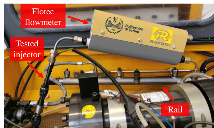
86 87 (b) The flowmeter with its external shell.
