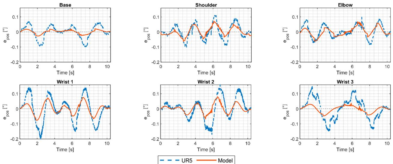
**Figure 8.** Mismatch between the target/set ( $q_{set}$ ) and the feedback/measured joints' angular positions ( $q_{FB}$ ) of the UR5 and the proposed model for the excitation trajectory for the excitation trajectory.
