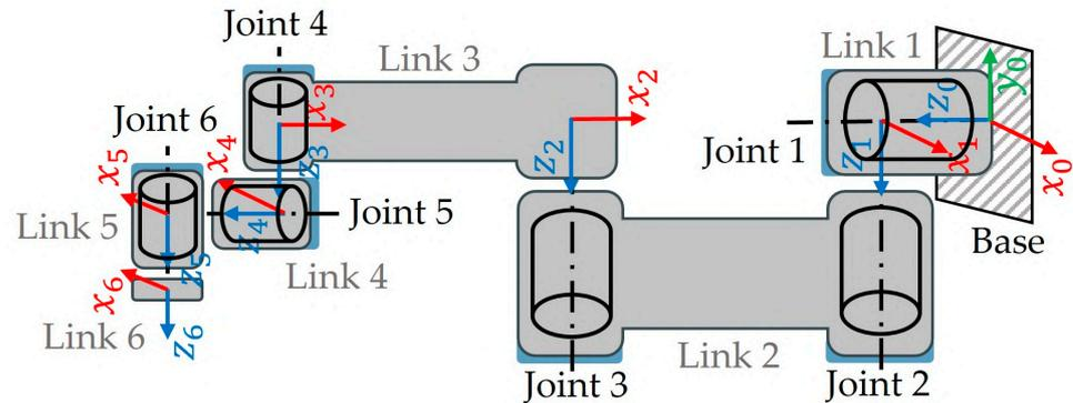
Figure 4. Schematic representation of the UR5 collaborative robot.
