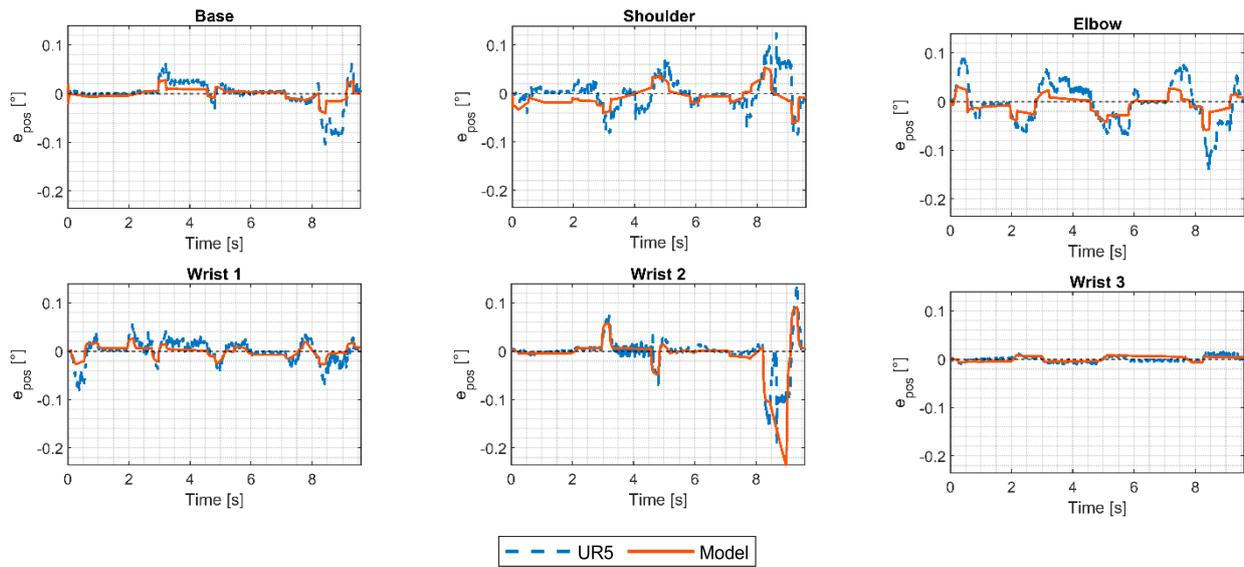
**Figure 11.** Mismatch between the target/set ( $q_{set}$ ) and the feedback/measured joints' angular positions ( $q_{FB}$ ) of the UR5 and the proposed model for the excitation trajectory for the pick-and-place trajectory.
