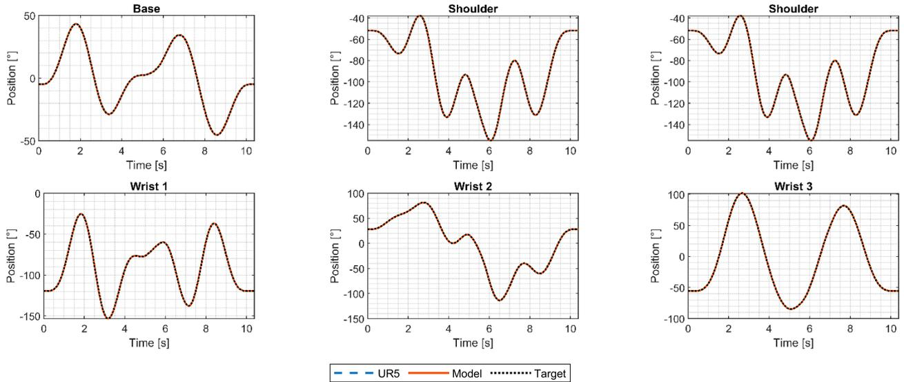
**Figure 7.** Comparison between the joints' angular positions measured from the UR5 and estimated through the proposed model ( $q_{FB}$ ) compared with the target/set ( $q_{set}$ ) values for the excitation trajectory.
