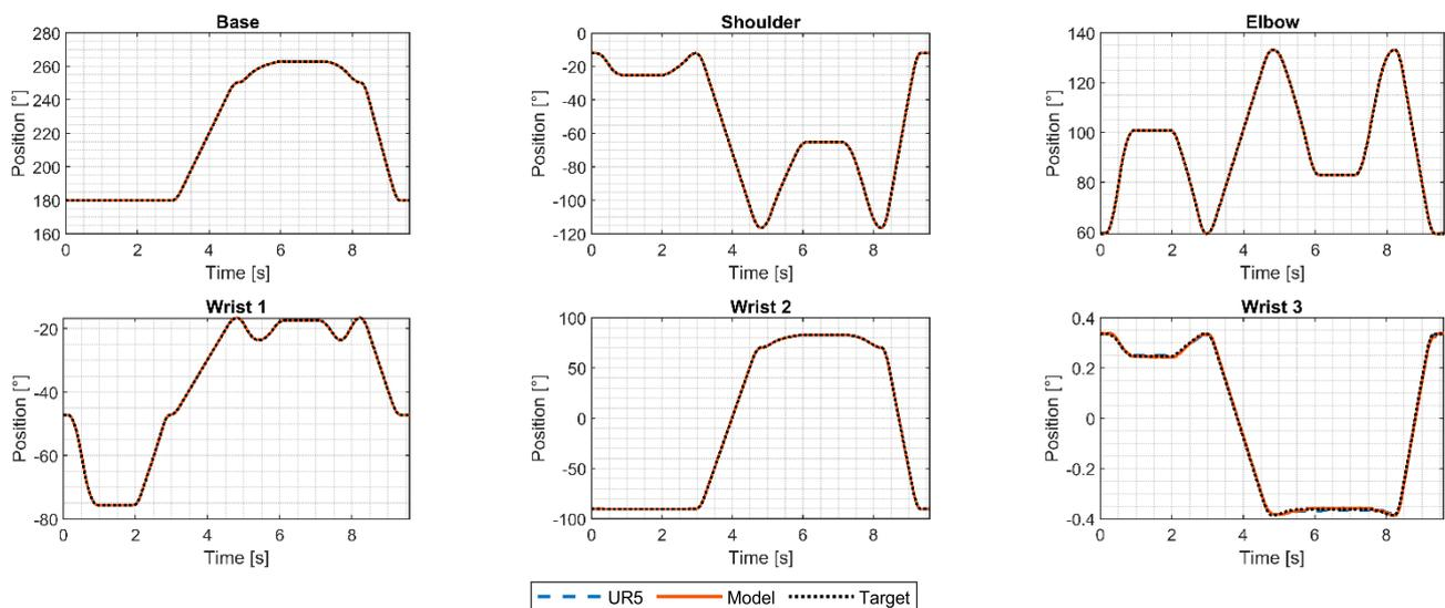
**Figure 10.** Comparison between the joints’ angular positions measured from the UR5 and estimated through the proposed model ( $q_{FB}$ ) compared with the target/set ( $q_{set}$ ) values for the pick-and-place trajectory.
