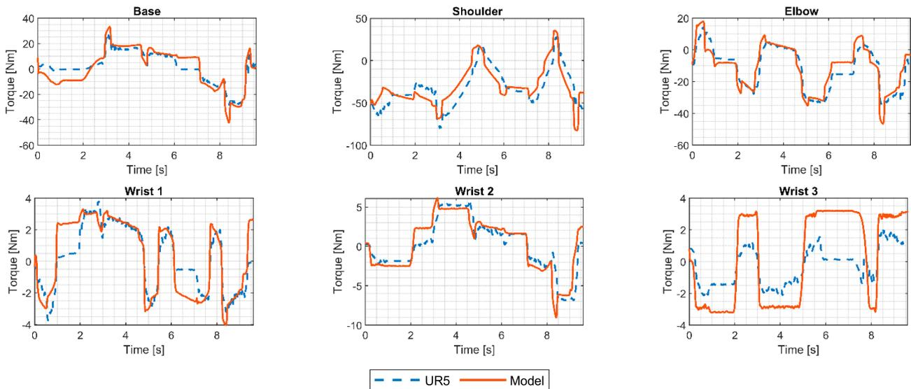
**Figure 12.** Comparison between the joints torques derived from the UR5 motor currents, the one estimated through the proposed model ( $i_{FB}$ ) for the pick-and-place trajectory and the one calculated by exploiting the Corke model.
