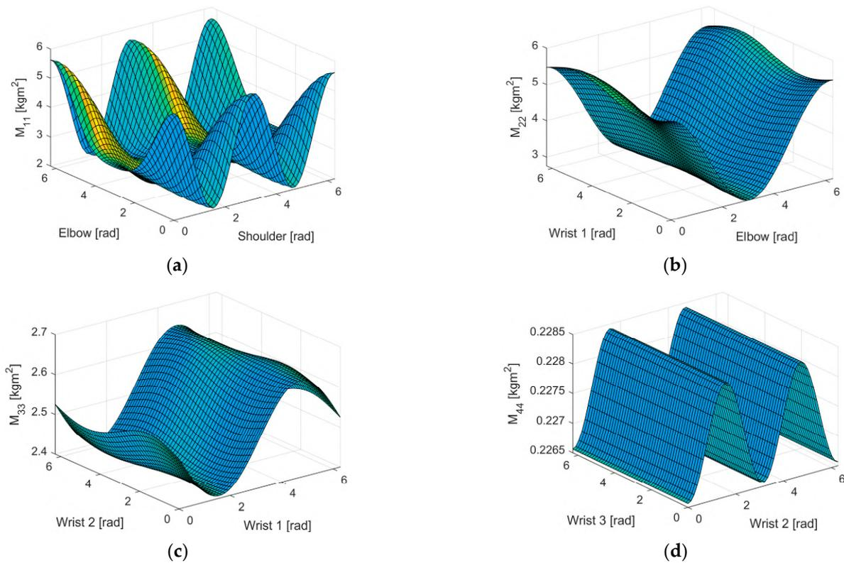
**Figure A2.** (a) Base inertia as a function of shoulder and elbow angles; (b) shoulder inertia as a function of elbow and wrist 1 angles; (c) elbow inertia as a function of wrist 1 and 2 angles; (d) wrist 1 inertia as a function of wrist 2 and 3 angles.
