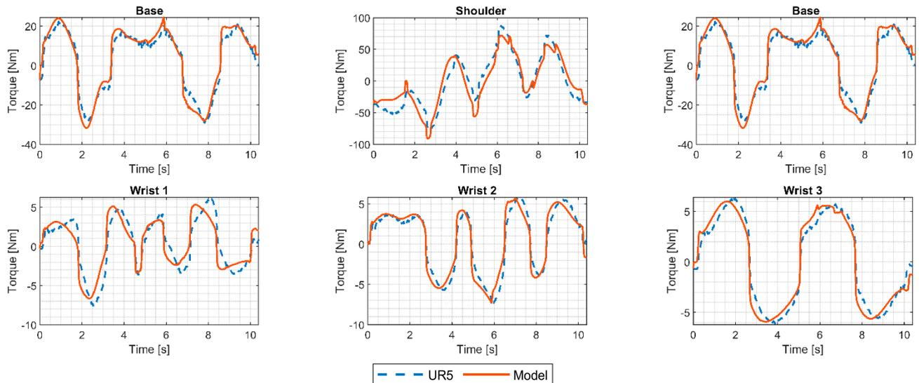
**Figure 9.** Comparison between the joints' torques derived from the UR5 motor currents, that estimated through the proposed model ( $i_{FB}$ ) for the excitation trajectory and that calculated by exploiting the Corke model.
