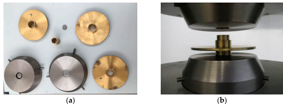
Figure 12. The specific cylinder with dedicated tools: brass cylinder and separators discs with dedicated extension poles (a); insert in hysteresisgraph joke (b).
