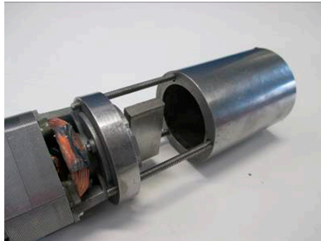
Figure 3. Proposed mechanical technique: impact mill.
