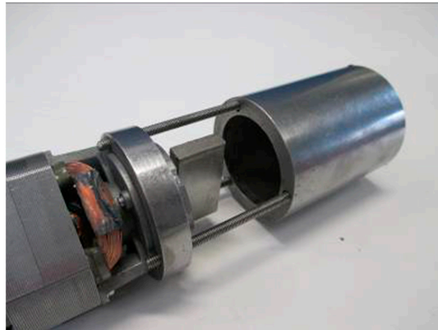
Figure 3. Proposed mechanical technique: impact mill.
