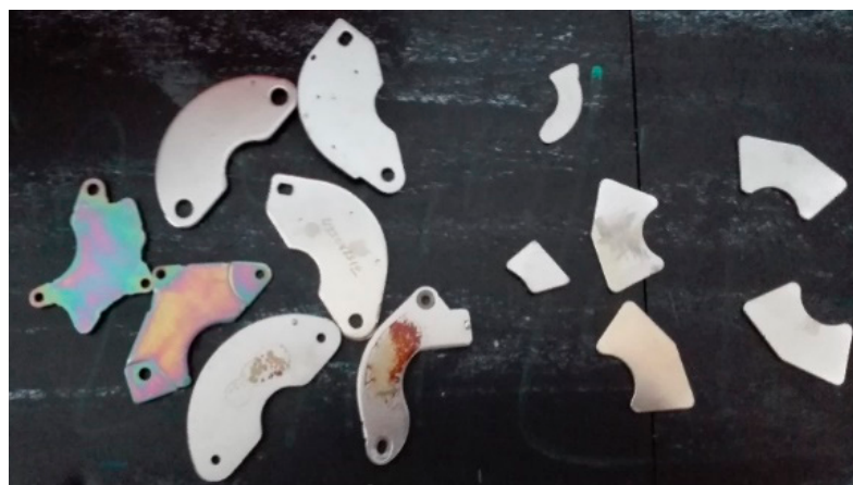
Figure 2. Different sizes of the recovered NdFeB magnets (some high- \mu shields on the left).
