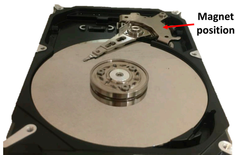
Figure 1. Hard disk drive with the magnet position.
