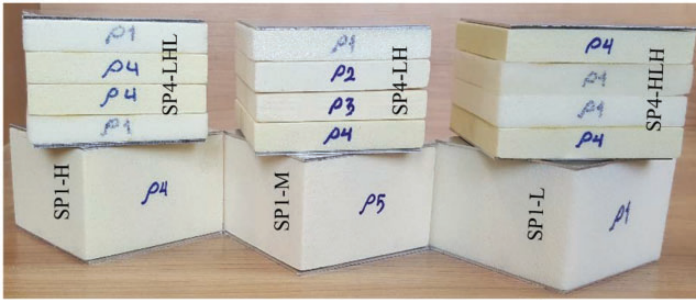
Figure 6. A number of sandwich panel samples with aluminum face-sheets and foam core (single layer and four layers).
