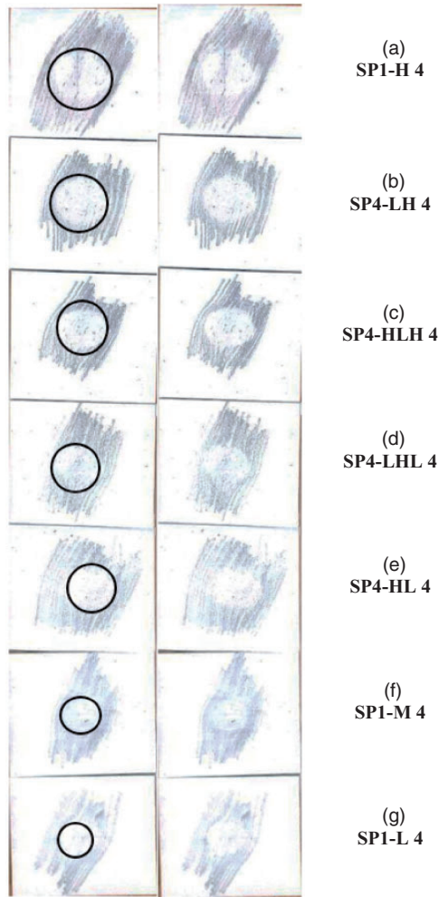
Figure 13. Papers with hachure for each of the seven types of sandwich structures at a speed of 275 m/s.
