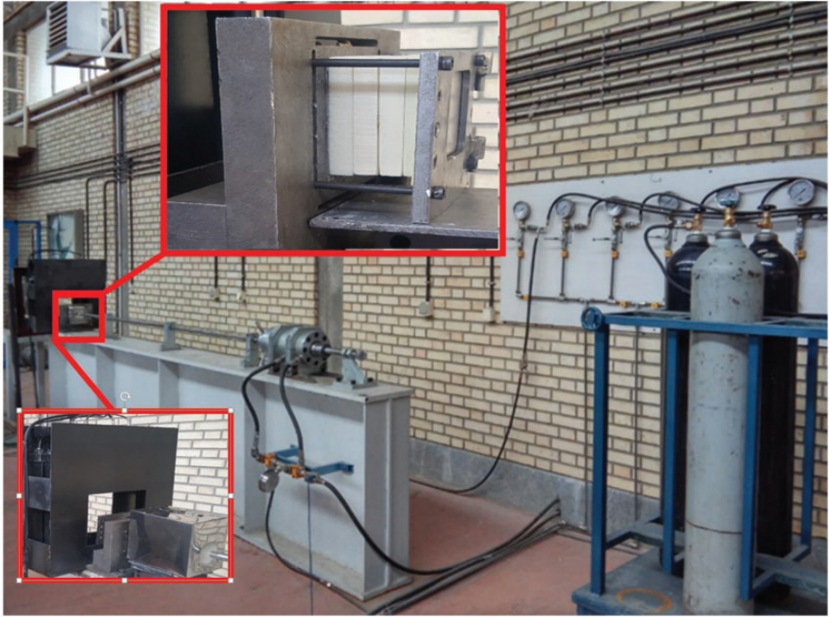
Figure 8. One-stage gas gun and the fixture.
