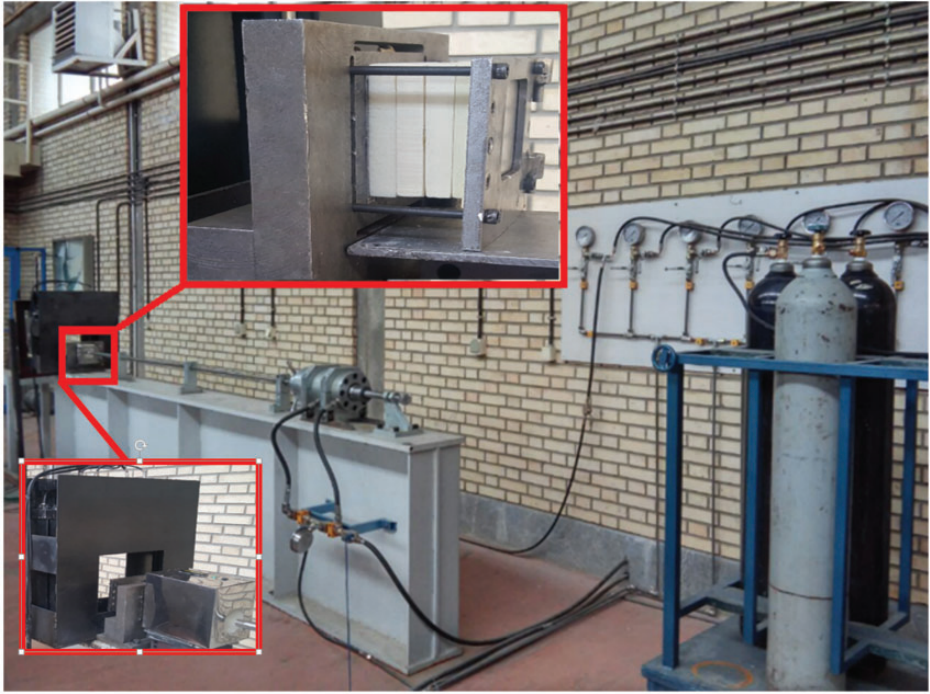
Figure 8. One-stage gas gun and the fixture.
