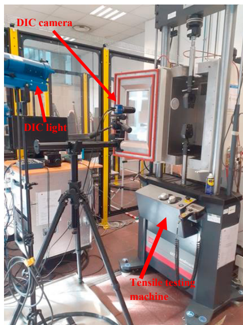
Fig. 4. Tensile testing machine and DIC configuration.
