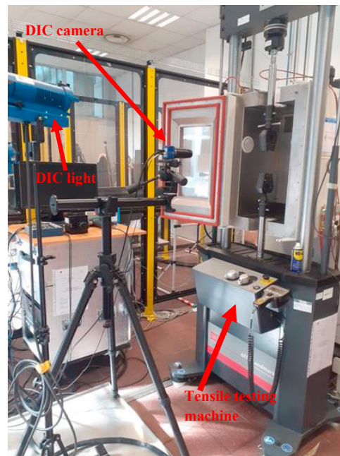
Fig. 4. Tensile testing machine and DIC configuration.
