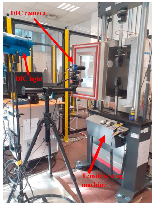
Fig. 4. Tensile testing machine and DIC configuration.
