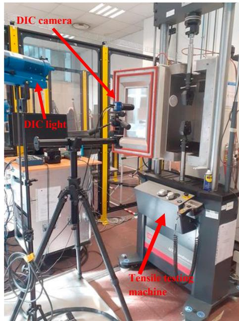
Fig. 4. Tensile testing machine and DIC configuration.
