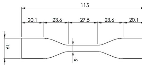
Fig. 1. Specimen geometry [30].
