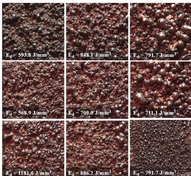
Fig. 3. Stereomicroscope images of the Cu – 0.5 % GNP.
