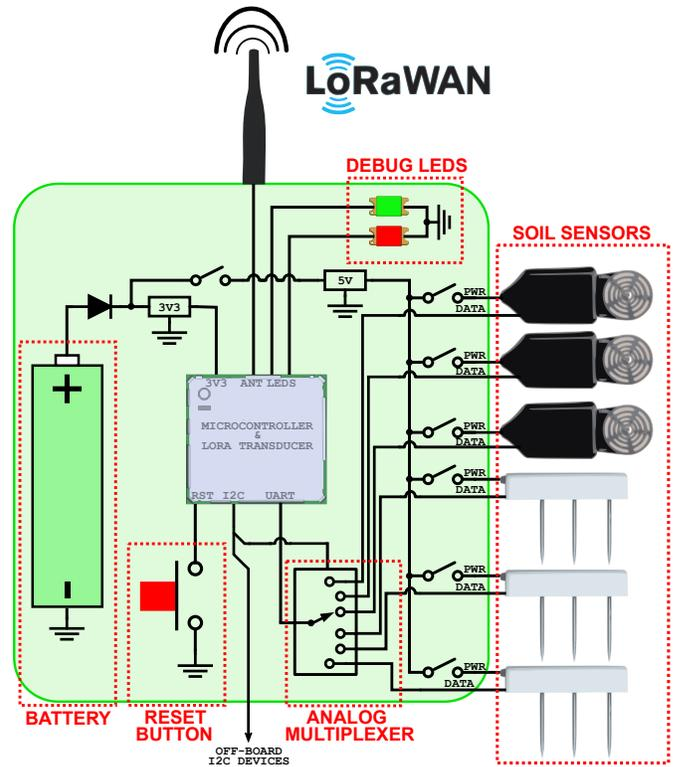
Fig. 2. LoRa plant water monitoring end node overview.
