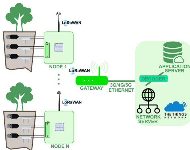
Fig. 1. Designed LoRa architecture water plant monitoring.
