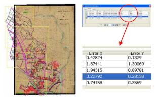
Figure 1. Geo-referencing of an historical map: on the right the discrepancies on check points expressed in pixel units
