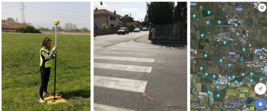
Fig. 12.2 GCPs materialized in the surveyed area and GNSS receiver (a). Natural point selected as GCP (b). Overall view of the GCPs (c). (Images from the 3D metric survey carried out by the Geomatics group of Politecnico di Torino)
