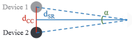
Figure 2: Evaluation of the minimum distance between the AVRS and sound source to obtain perceptually coherent AV scenes.
