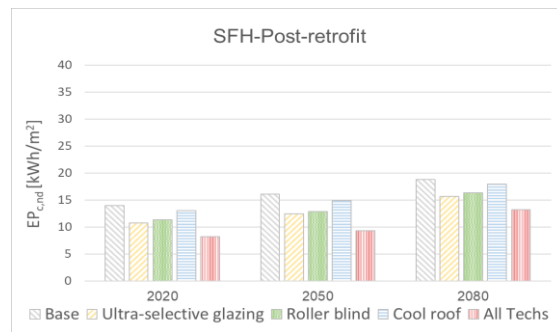
Fig. 3 – Thermal energy need for space cooling (June/July/August) in 2020, 2050, and 2080 for post-retrofit building
