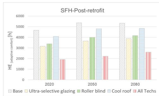
Fig. 7 – Weighted hours of exceedance (June/July/August) in 2020, 2050, and 2080 for post-retrofit building, in free-floating condition
