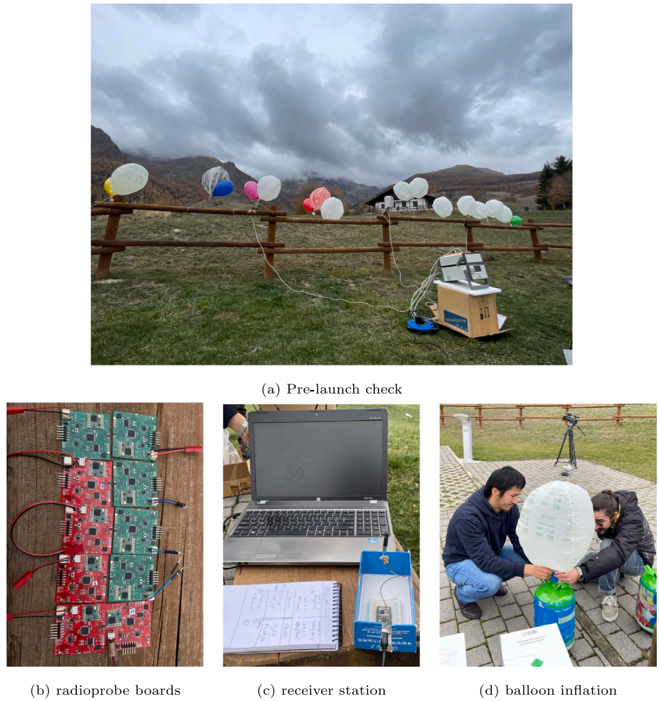
Fig. 16. Experiment setup at OAVdA , St. Barthelemy, Aosta, Italy, on November 3, 2022. (a) The radiosondes during pre-launch calibration with INRIM reference instrumentation. (b) Prepared radioprobe electronic boards. (c) A ground station connected to the laptop PC. (d) Balloon preparation for radiosonde assembly.
