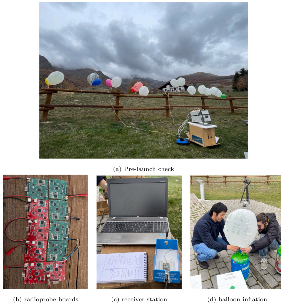
Fig. 16. Experiment setup at OAVdA , St. Barthelemy, Aosta, Italy, on November 3, 2022. (a) The radiosondes during pre-launch calibration with INRIM reference instrumentation. (b) Prepared radioprobe electronic boards. (c) A ground station connected to the laptop PC. (d) Balloon preparation for radiosonde assembly.
