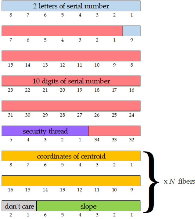
Fig. 5. Proposed encoding scheme, with bit size for each field. N is the number of fibers found in the banknote.
