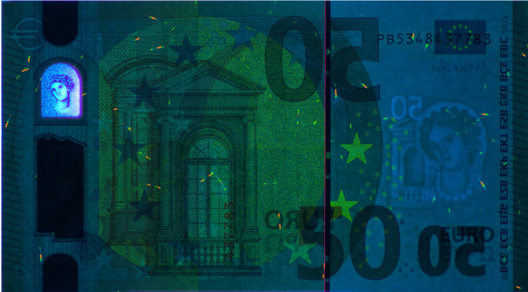
Fig. 3. Highlight of fibers and security thread in the ultraviolet image of a € 50 banknote.
