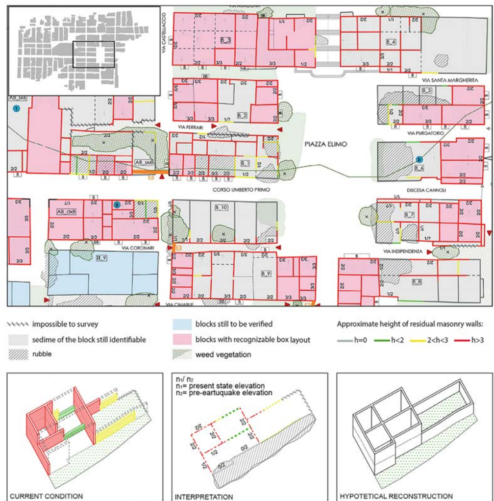
Figure 10. The “present state map” assembles data on current conditions using graphic conventions to collect multilayered information (authors’ drawing).
