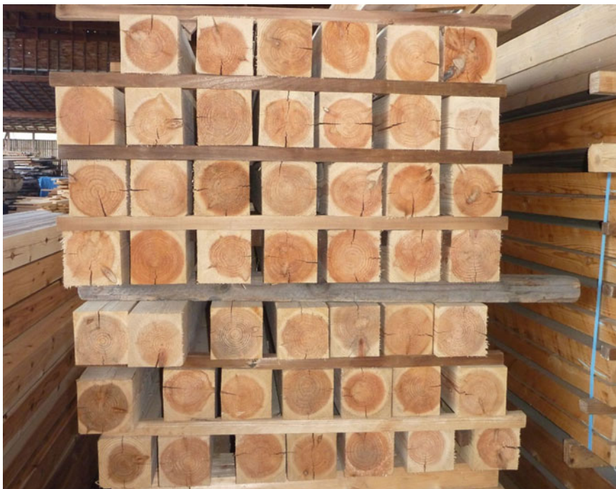
Fig. 33.2 Timber dried at low temperatures in a greenhouse at Kitokuras sawmill (Kagawa prefecture). Photo Andrea Bocco Guameri
