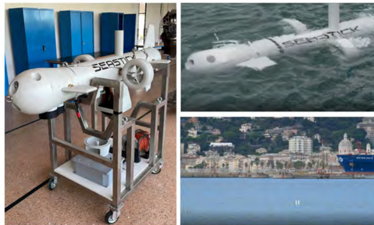
Figure 1. AUV equipped with sensors for seabed monitoring and at sea during the pilot test.
