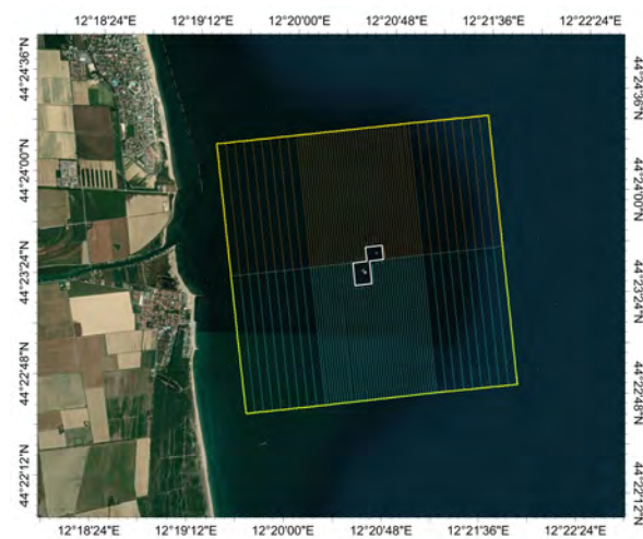
Figure 5. Planned trajectory of the AUV for the survey. The two sub-trajectories are represented by the orange and light-blue lines.
