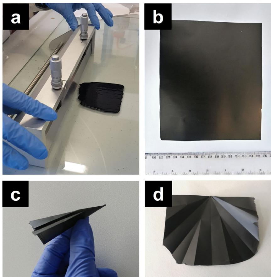
**Fig. 1 Scalable GO membrane.** **a** Production of GO membrane by Dr. Blade technique. **b** Scalable GO membrane of a dimension of 14.5 cm × 14.5 cm with a ruler in cm placed on the bottom. **c** Origami figure made of a GO membrane to show its mechanical resistance. **d** GO membrane after undoing the origami figure.
