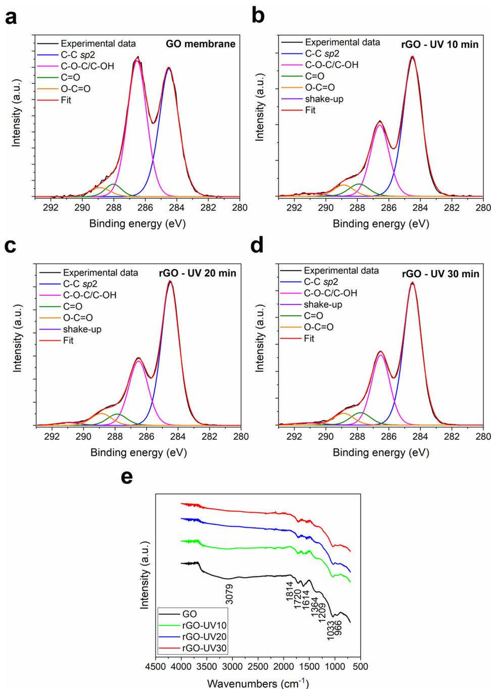
**Fig. 6** High-resolution C 1s XPS spectra of GO membranes. **a** As-prepared, **b–d** after UV-light irradiation for 10, 20, and 30 min. **e** Evolution of the IR spectrum of GO after UV-light irradiation at different times.
