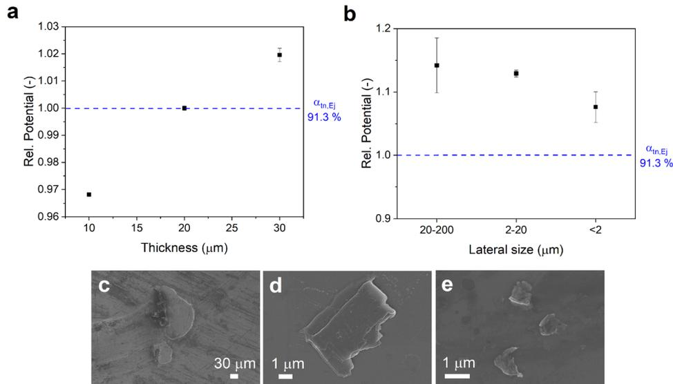
**Fig. 9** Permselectivity of GO membrane in NaCl 0.1/0.5 M as a function of. **a** thickness **b** lateral size. Error bars correspond to the standard deviation of each measurement. Graphene oxide flakes were obtained after centrifugation at **c** 1000 rpm, **d** 2000 rpm, and **e** 3000 rpm.
