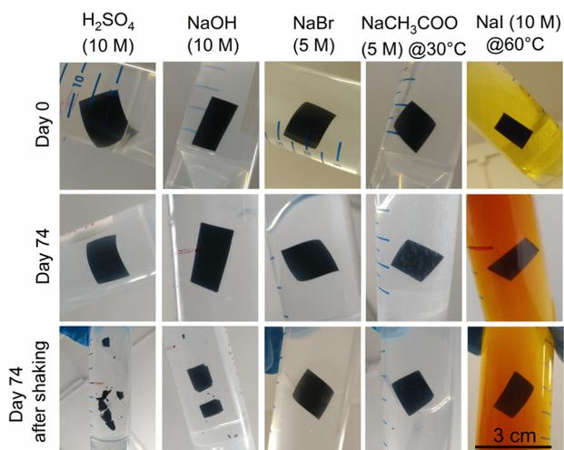
**Fig. 2** Chemical stability of GO-20 membrane under different solutions. Membranes were tested during 74 days under static and dynamic conditions in  $\text{H}_2\text{SO}_4$  10 M, NaOH 10 M, NaBr 5 M,  $\text{NaCH}_3\text{COO}$  5 M, and NaI 10 M.
