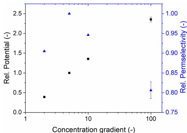
**Fig. 8 Normalized potential and permselectivity of GO-20 membrane under different concentration gradients.** A fixed concentrated solution of KCl 1 M was selected. Error bars correspond to the standard deviation of each measurement.
