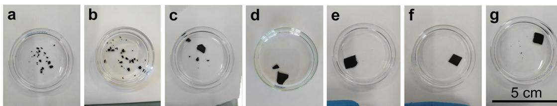
**Fig. 3 Mechanical stability of thin composite membranes of a dimension of 1 cm<sup>2</sup> in water. a** GO-10, **b** GOPVDF-10, **c** GOPEO-10, **d** GOchit-10, **e** GOPVA-10, **f** GOPVP-10, and **g** GOSPEEK10-10.
