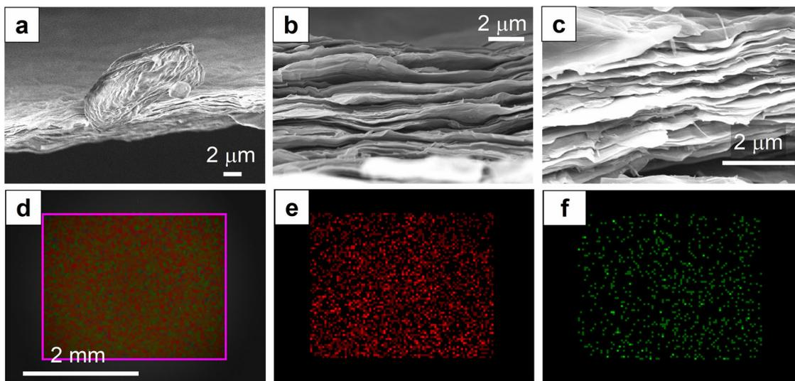
**Fig. 5 Cross-section of composite membranes. a** GOPVA-20 with a PVA agglomerate on its structure. **b** GOPVP-20 membrane. **c** GOSPEEK20-20. EDX mapping of S and Na in the GOSPEEK20-20 membrane matrix. **d** S and Na, **e** S, and **f** Na.
