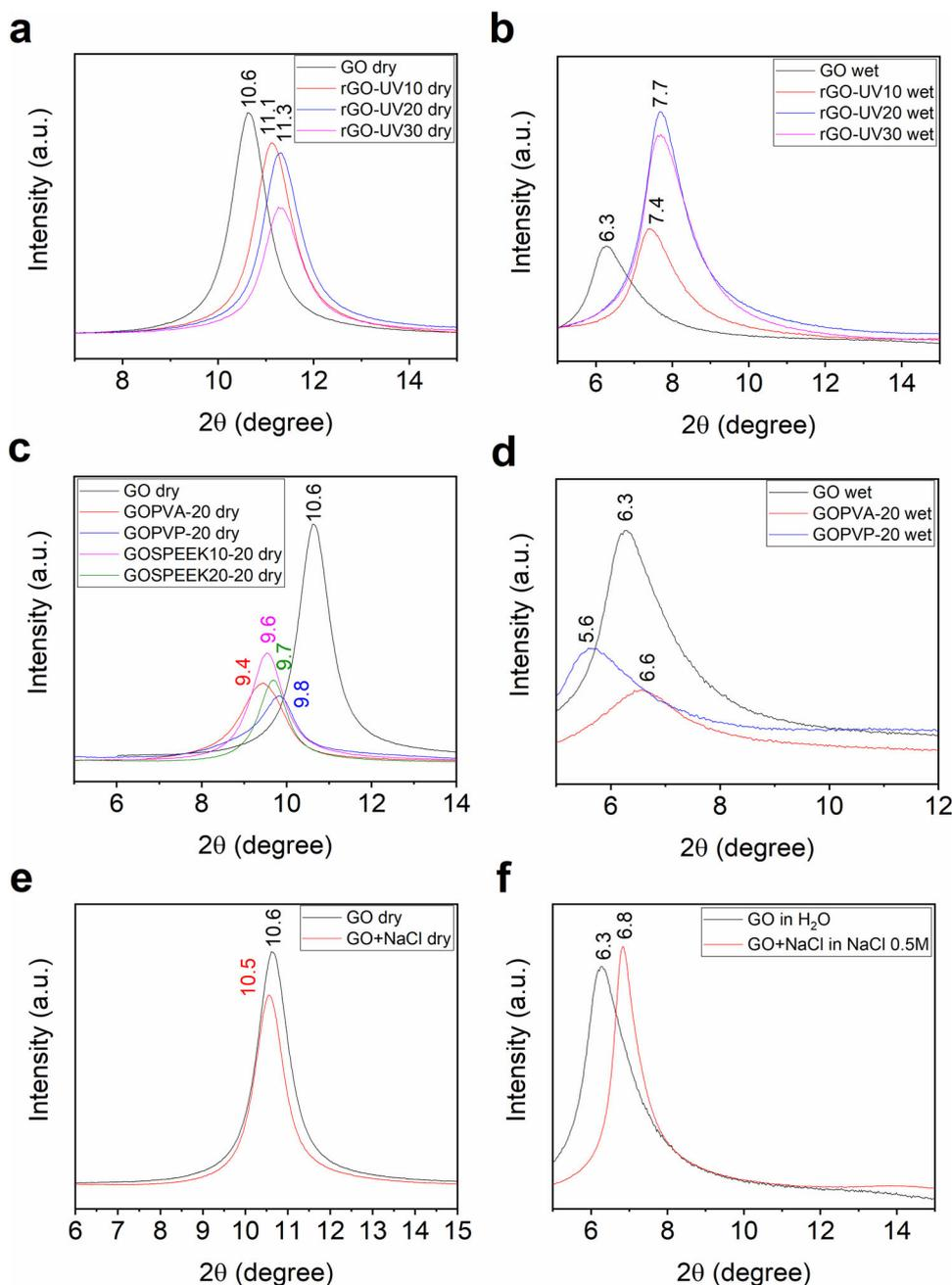
**Fig. 7** XRD measurement of GO membranes reduced at 0, 10, 20, and 30 min. **a** Dry, **b** wet states, composite membranes in **c** dry **d** wet states, and GO membrane and GO with NaCl salt inside the channels in **e** dry **f** wet states.
