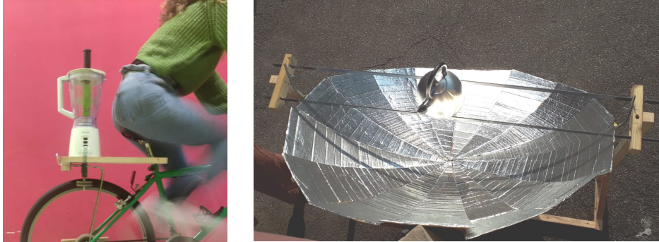
Fig. 2. Bike-blender and parabolic solar oven built in the experimental laboratory.
