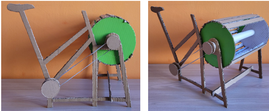
Fig. 1. Model of pedal powered cassava peeling machine. Courtesy of Giovanni Artioli, Cesare Barbera, Matilde Cais, Flavia Coli, Pietro Ghibaudo and Serafini Emma students.
