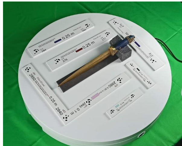
Figure 5. Scale bars and museum artefact positioning on the rotating platform
