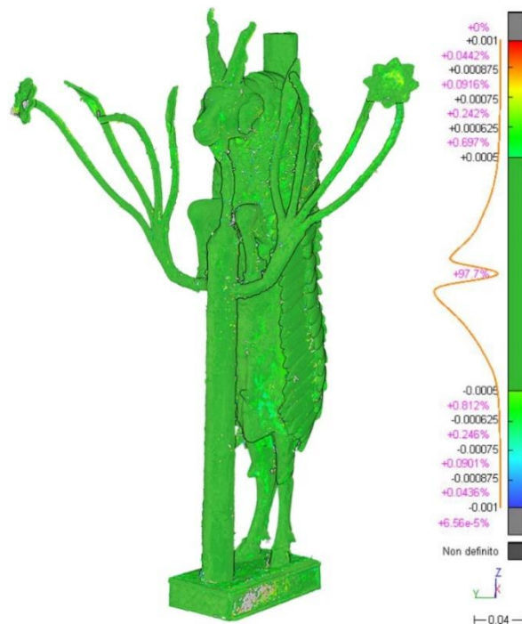
Figure 10. Distance analysis between the photogrammetric and laser scanning point clouds of the ram in a Thicket artefact, highlighting an average discrepancy lower than \pm 0.5 mm.
