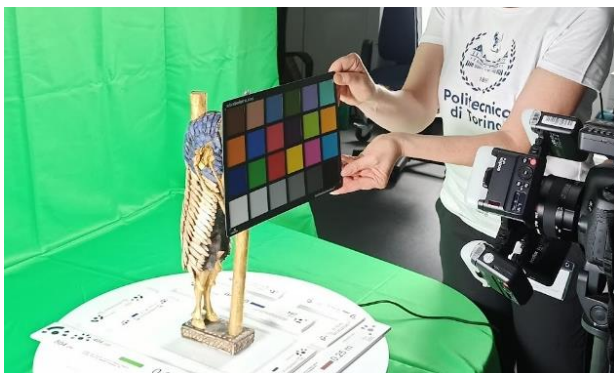
Figure 4. Preliminary acquisition of a radiometric calibration panel for each different acquisition configuration.
