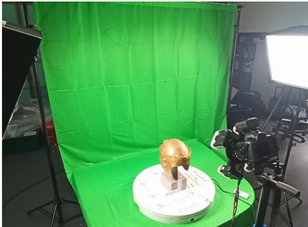
Figure 3. 3D close-range photogrammetric survey general set-up, including green screen, artificial LED lights, DSLR camera mounted on a tripod, four flashes mounted on the camera lens ring, and rotating platform.
